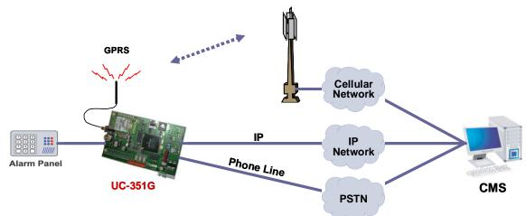
The IP path uses highly encrypted messaging over a corporate IP WAN or broadband internet connection such as ADSL, Cable Modem or Wireless (eg WiMax or HSDPA). The GPRS link is implemented as a secure VPN. The unit supports a range of interfaces to intruder alarm systems, including dial-capture, parallel inputs and the ASIAL (SecuriteI<sup>™</sup>) serial interface, both TTL and RS.232 connections are supported. The inbuilt dialler can deliver alarms received over the serial interface.
